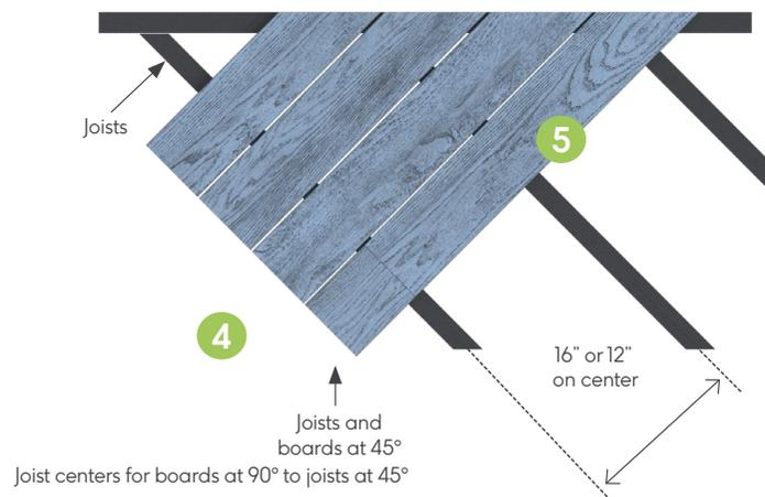
**Top tip:** The boards are 141" long, reduce the joist centers to 15 1/2" and 11 1/2" respectively to reduce wastage.
