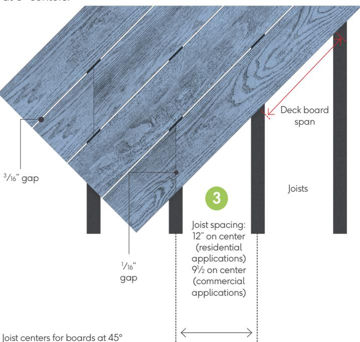
For laying boards 45° to the joist, reduce the joist centers to 12" for residential and 10" for commercial use. (3) Alternatively turn the joists round to be at 90° to the board direction (4) as this is less wasteful of material and time. If you need to cut Millboard decking down along the length, reduce the joist centers accordingly. A minimum of three joists is required for any cut boards. (5)
