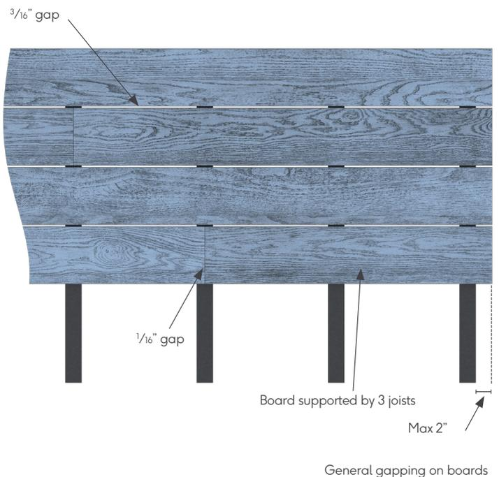
A gap between the boards smaller than  $\frac{3}{16}$ " can lead to dirt build-up and can prevent drainage between the boards. It can also lead to the boards rubbing against each other causing a squeaking noise. Gaps bigger than  $\frac{1}{4}$ " can result in items falling through or getting stuck, such as high heels, children's fingers, rings, keys, etc., as well as exposing more of the joist which is often not the desired look
