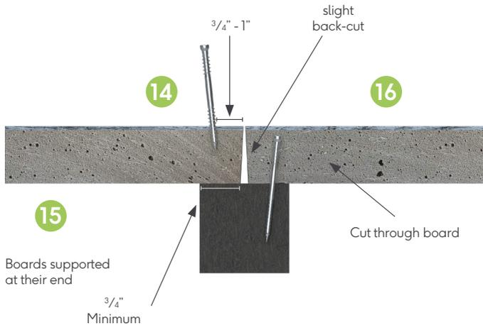
Cuts must always be positioned over the joist. We recommend that all ends are squared off with a slight back cut of around 2-3 degrees before they're installed (16). This back-cut makes it easier to adjust butt joints if required, by carefully running a handsaw along the gap to make the butt joint square and evenly gapped.
