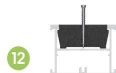
Failure to use our Durafix screws with the bit provided or not installing according to these guidelines may invalidate the warranty and affect the overall look of the deck. Two screws per board should be used where the board crosses a joist. Use three at the ends of the boards. (13)
