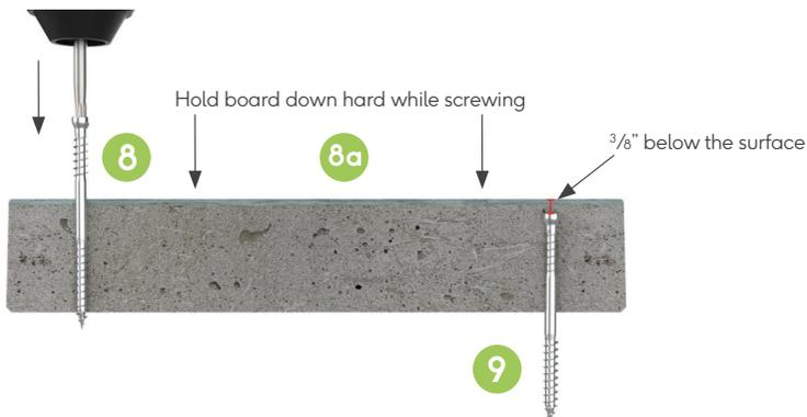
Millboard decking can be installed onto lumber joists using Durafix 60mm (2 3/8") screws. (10)
