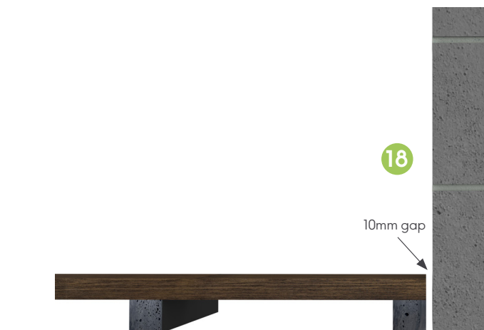
Gap between boards and solid surfaces
