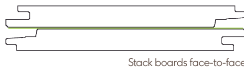
Stack boards face-to-face
